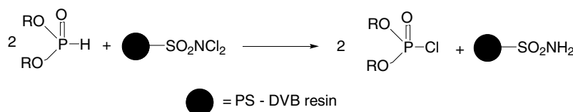
Scheme 1. Dialkyl chlorophosphates prepared from dialkylphosphites using the polystyrene divinylbenzene (PS-DVB) bound reagent.
